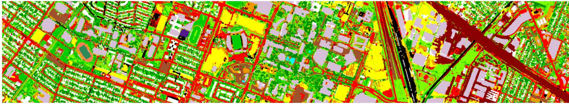
Fig. 6. Final classification result using two random forests, MMS correction, and post-classification segmentation.
