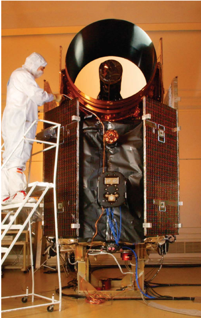
Fig. 5. Photograph of the GLAS upon lidar integration with ICESat at Ball Aerospace and Technology Corp.
