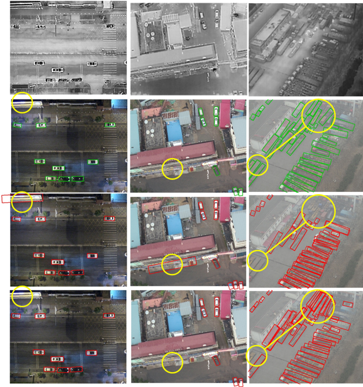
Fig. 8. Subjective diagram of test results. The rows from top to bottom are labeled optical images, baseline detection results, and the results of the FFODNet.
