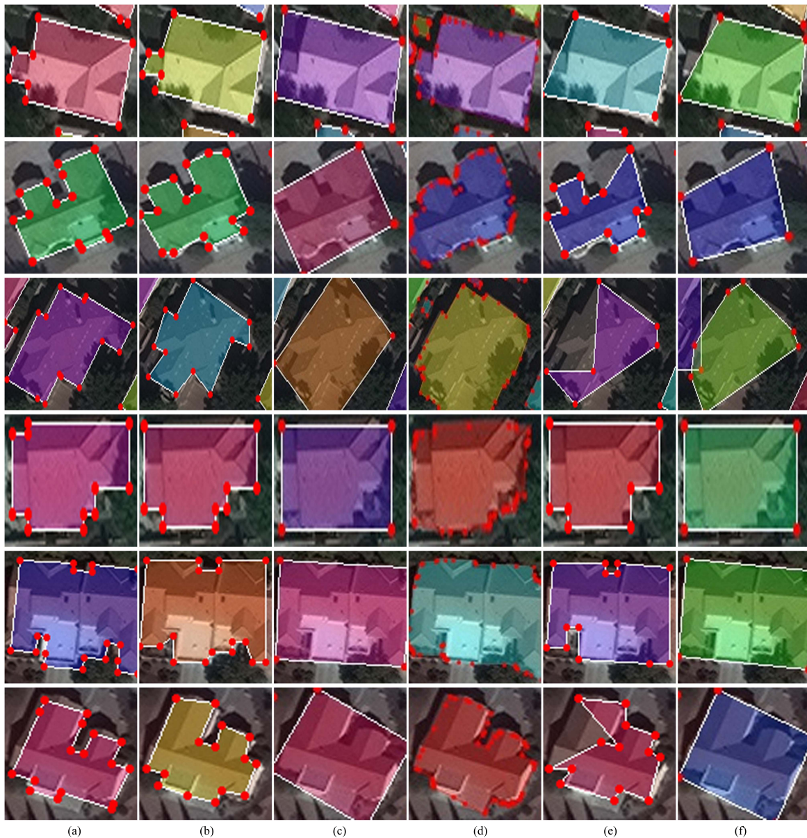
Fig. 9. Qualitative results on SpaceNet (Las Vegas). Column (a): GT. Column (b)–(f): Building footprint extraction of our method, Mask RCNN, FFL, PolyMapper, and PANet.
