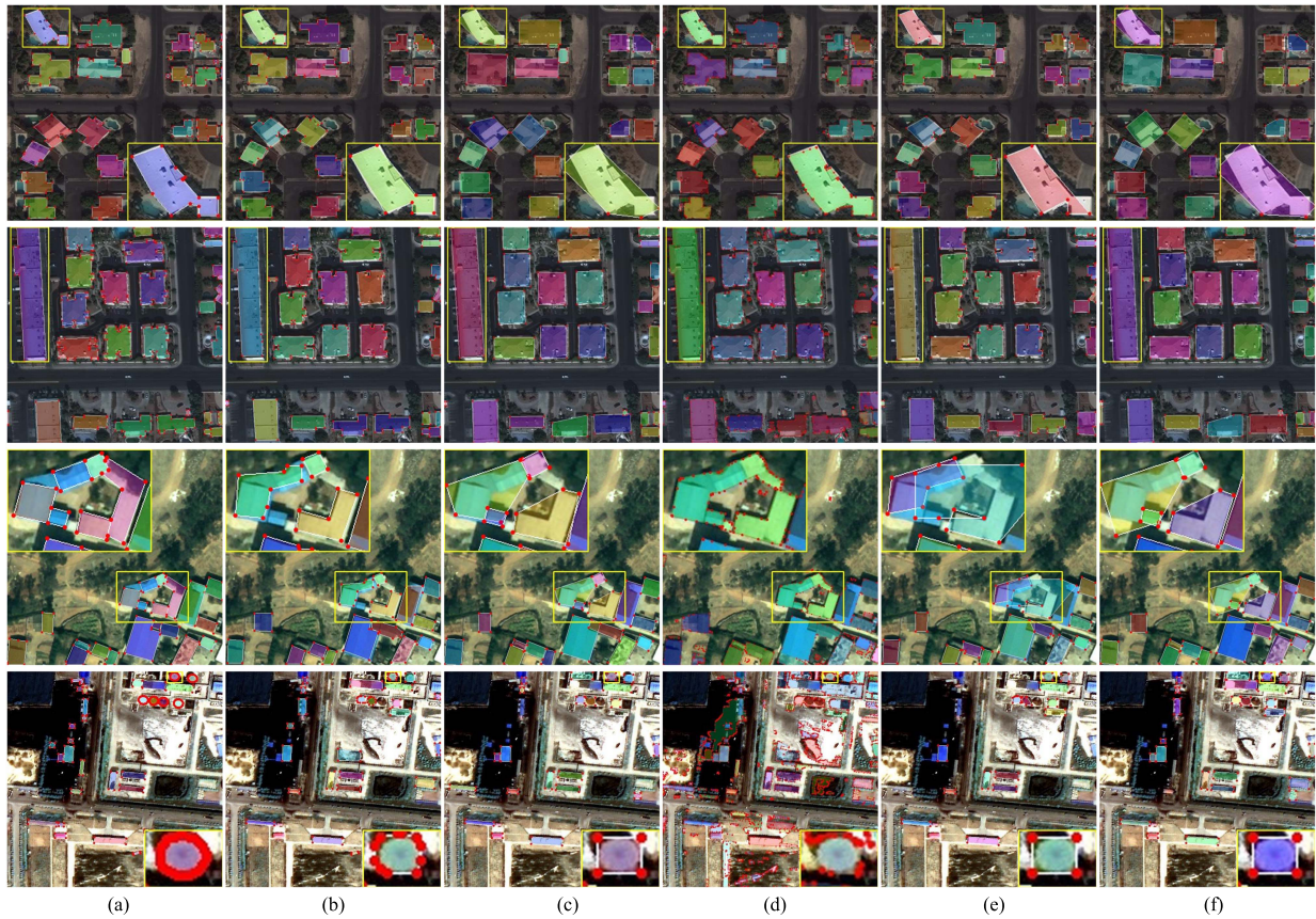
Fig. 7. Qualitative results on three building test datasets. We underline and scale up the large and complex buildings for convenient comparison. Column (a): Corresponding ground truth. Column (b)–(f): Building footprint extraction results of our method, Mask RCNN, FFL, PolyMapper, and PANet, respectively. Row 1st and 2nd: SpaceNet (Las Vegas). Row 3rd: CNDData. Row 4th: 5M-Building.
