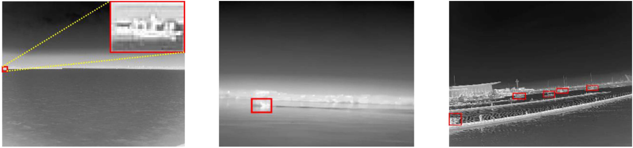
Fig. 1. Example images of infrared ships. We give three infrared ship targets in Fig. 1, the first image shows a weak target under the effect of long-range imaging, the second image shows a target near the harbor under low contrast, and the third image shows multiple targets under the complex background near the harbor. Ship targets are indicated by red borders and the first image is zoomed in at the top right corner.
