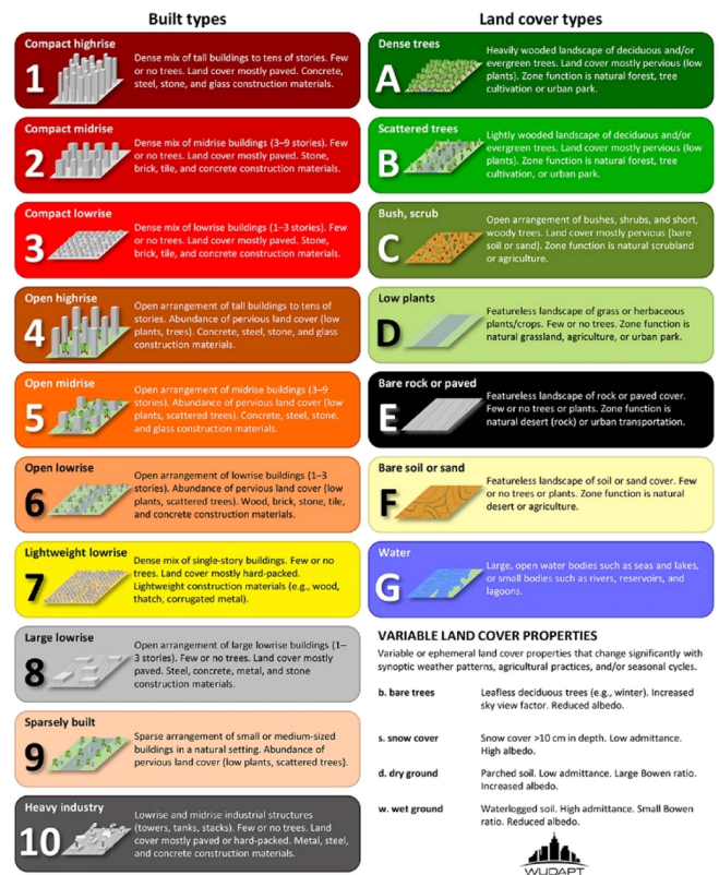
Fig. 1. Built types (1–10) and land-cover types (a)–(g) LCZs defined by Demuzere et al. [3].
