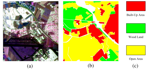
Fig. 7. ESAR Oberpfaenhofen dataset and its color code. (a) Pauli-RGB image. (b) Ground truth map. (c) Legend of the dataset.
