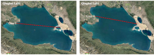
Fig. 12. Case 1 and Case 2 specular reflection point trajectories, ice(left), lake(right).
