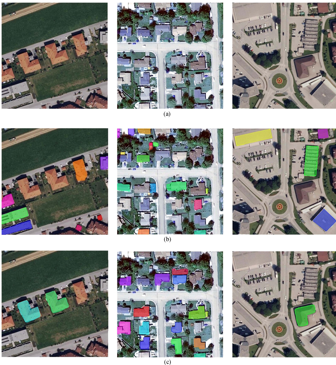
Fig. 18. Comparison of sample ablation results based on a subset of geometric features. (a) is the original image. (b) Test results for model training using only a subset of rectangular building rooftop samples. (c) Test results for model training using only a subset of L-shaped building rooftop samples. (a) Original image. (b) Only rectangle image. (c) Only L roof.
