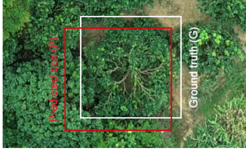
Fig. 9. Intersection over union of the ground truth and prediction bounding box.
