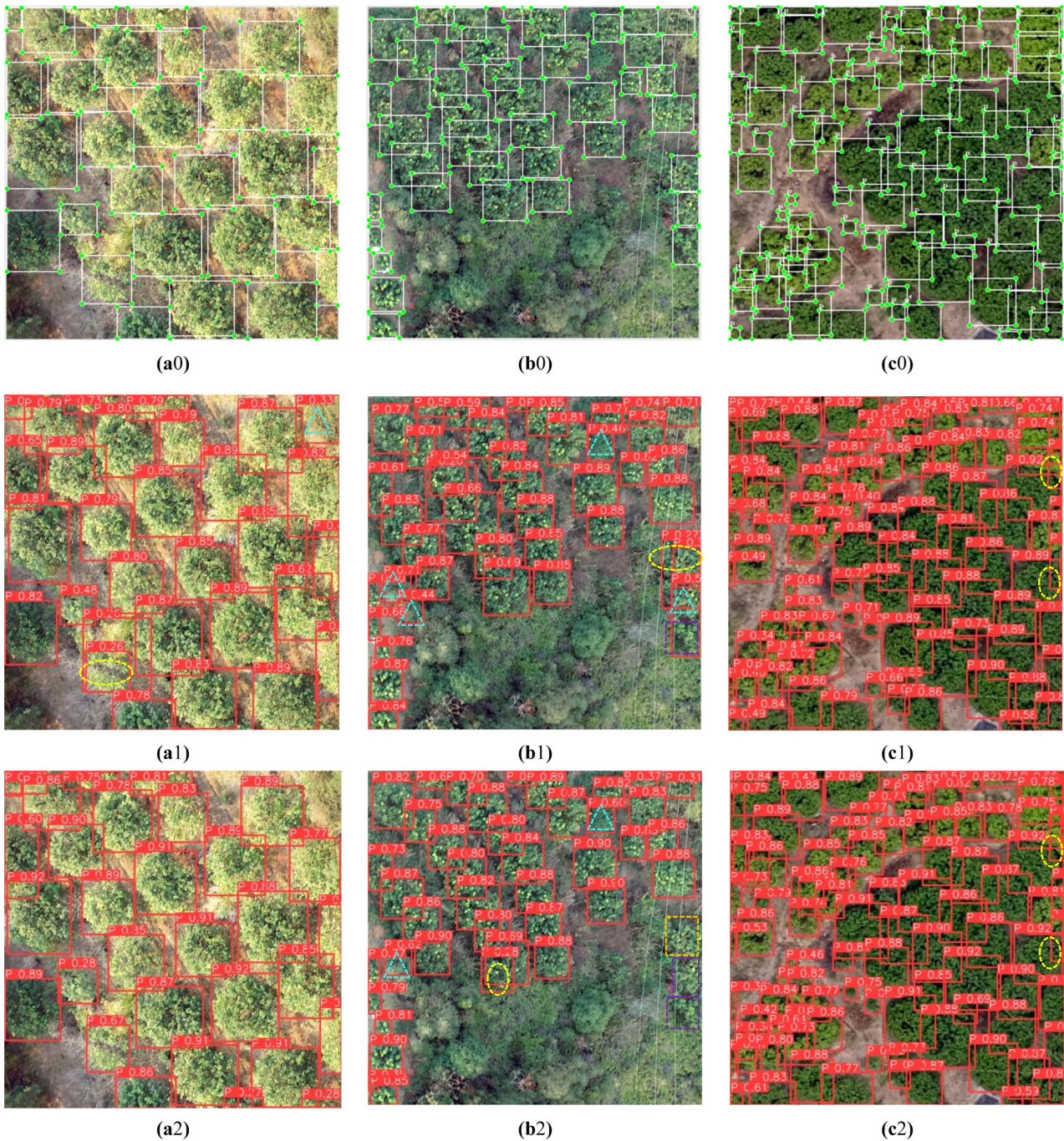
Fig. 17. Clip images overlaid with the ground truth boxes (a0, b0, and c0) and the detected IPT boxes and confidence scores predicted by YOLOv5s (a1, b1, and c1) and YOLOv5s-CA (a2, b2, and c2), respectively. (a) IPTs in sparse alignments. (b) IPTs in dense alignments interspersed with other trees. (c) IPTs in a dense and random distribution. Images (a) and (b) were selected from site B in the town of Sanxiang, and image (c) was deliberately selected from the other orchard near site A in the town of Shishan, Meizhou. These three images were not fed into the models for training. Note: White rectangles denote the manually labeled ground truth boxes, red rectangles denote the predicted bounding box with the class P and confidence score shown above it, brown rectangles denote the undetected IPTs, yellow ellipses denote the repeatedly overlaid IPTs, and cyan triangles denote the falsely predicted IPTs.
