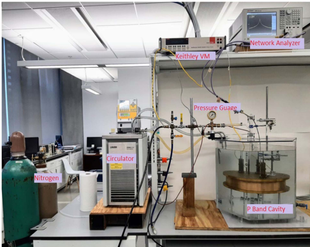
Fig. 3. Experimental setup for the measurement of the dielectric constant of sea water at P -band. The system is the same as used at L -band [4] except for the resonant cavity, which is larger and resonant at 0.707 GHz.
