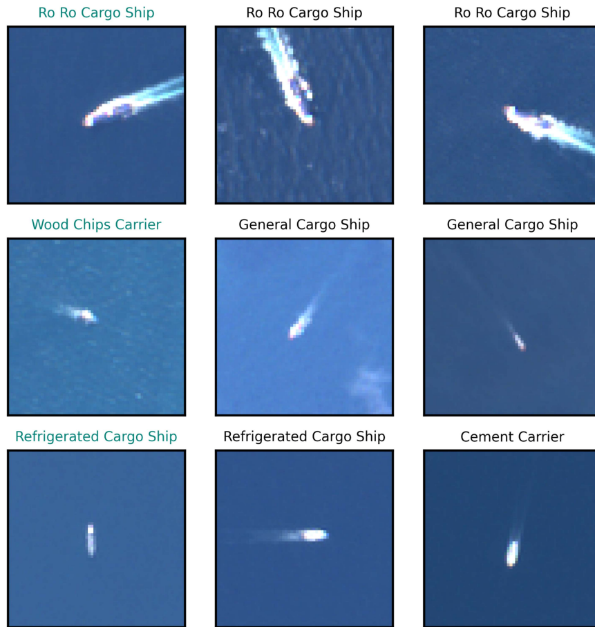
Fig. 9. Example of classification using similarities for three ships. The first column contains the input ship and ground truth AIS type. The following two images are the most similar ships in the reference set.
