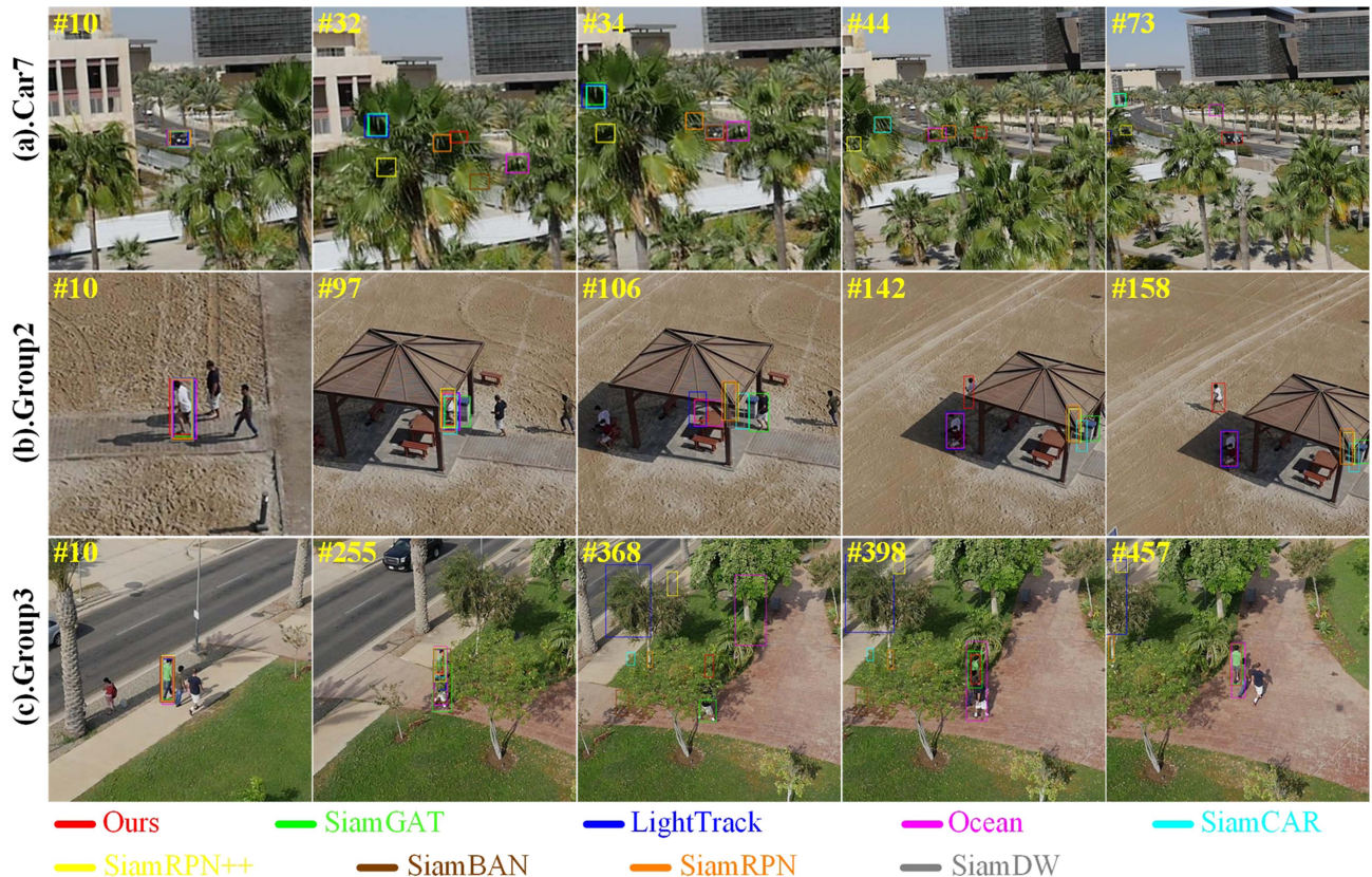
Fig. 8. Visual tracking results on UAV123. The figure consists of three subsequences, corresponding to challenges posed by frequent short-term occlusion, long-term complete occlusion, and masked coverage occlusion.
