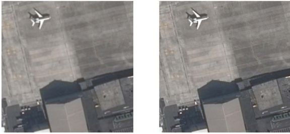
Fig. 2. Side-by-side comparison of iSAID-derived training data, with the low-resolution input image ( 242 \times 242 pixels) on the left and the high-resolution target image ( 1210 \times 1210 pixels) on the right.
