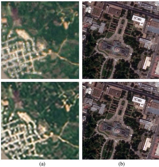
Fig. 16. Input images (top) and the results (bottom) of applying the SISR approach on (a) 30-m GSD imagery from Landsat 8 and (b) 1-m GSD imagery from satellite JL-1.
