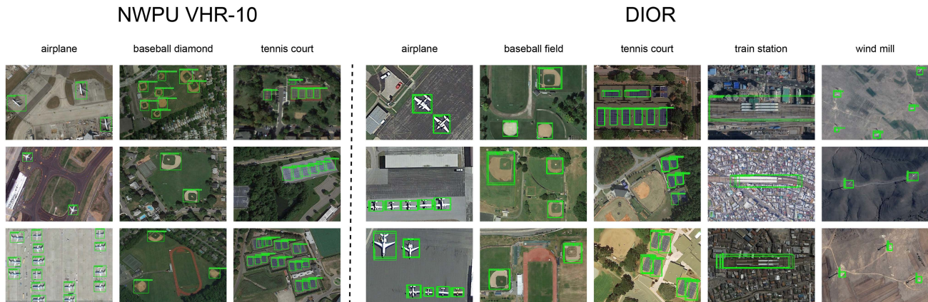
Fig. 5. Few examples of few-shot detection outcomes. (Left) Results of detection using a 10-shot setting on the novel classes in the NWPU VHR dataset. (Right) 20-shot detection results for the novel classes in the DIOR dataset.
