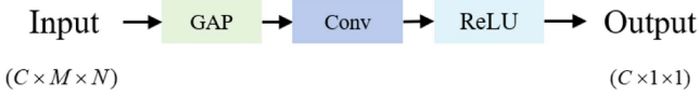
Fig. 7. Structure diagram of the global feature extraction layer. The input size of the global feature extraction layer is c \times m \times n , where c denotes the feature channel dimension, and m \times n denotes the size of the feature map. After the GAP processing, the size of the features becomes c \times 1 \times 1 . At this time, there is only one feature value for each channel, and this feature value is calculated from the global features of each channel.
