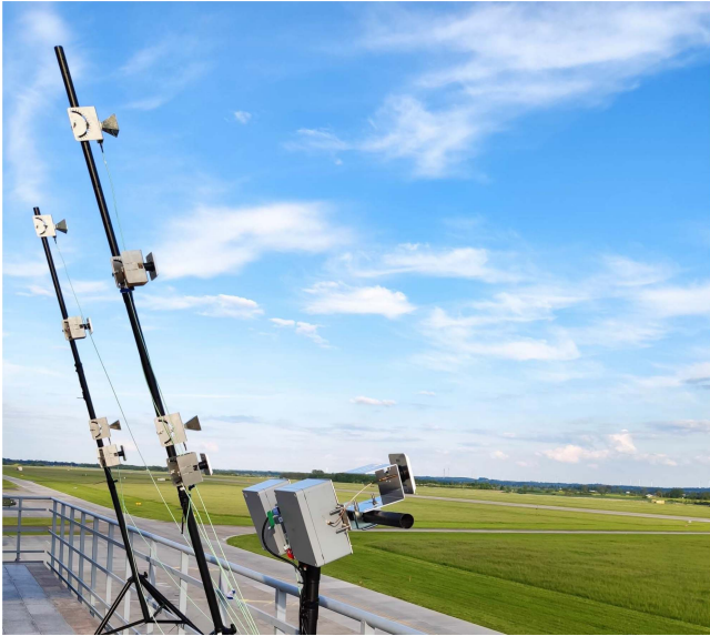
Fig. 12. Antennas setup of the X-band active radar demonstrator.
