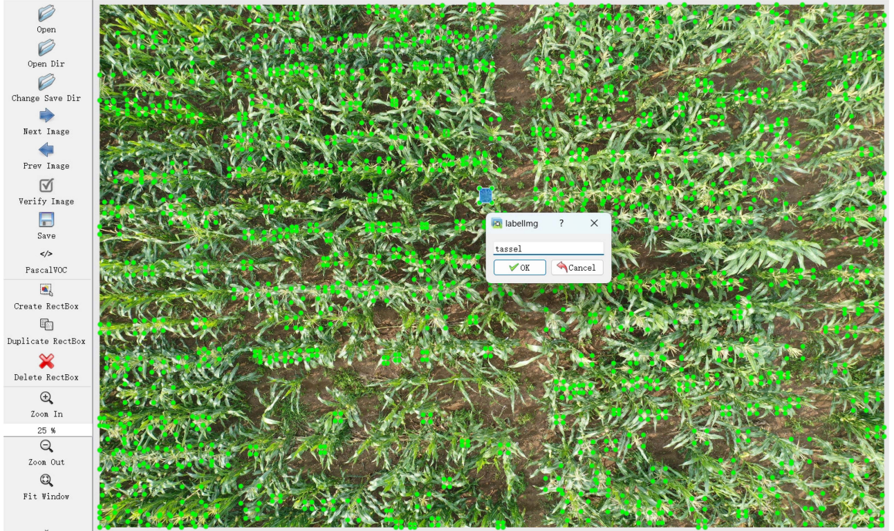
Fig. 1. Example of bounding box annotation in the MTC-UAV dataset, with reference to existing point annotations during the labeling process.
