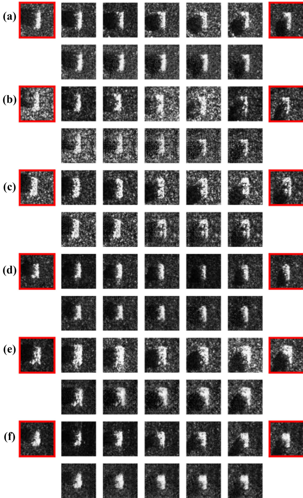
Fig. 6. Samples of real SAR and images generated by O2S+PD(S) with depression angle 15^\circ of (a) 2S1, (b) BRDM2, (c) BTR60, (d) T62, (e) T72A07, and (f) ZSU234. In each panel, the upper row is real SAR and lower row is generated images. Those with red frame are training samples.
