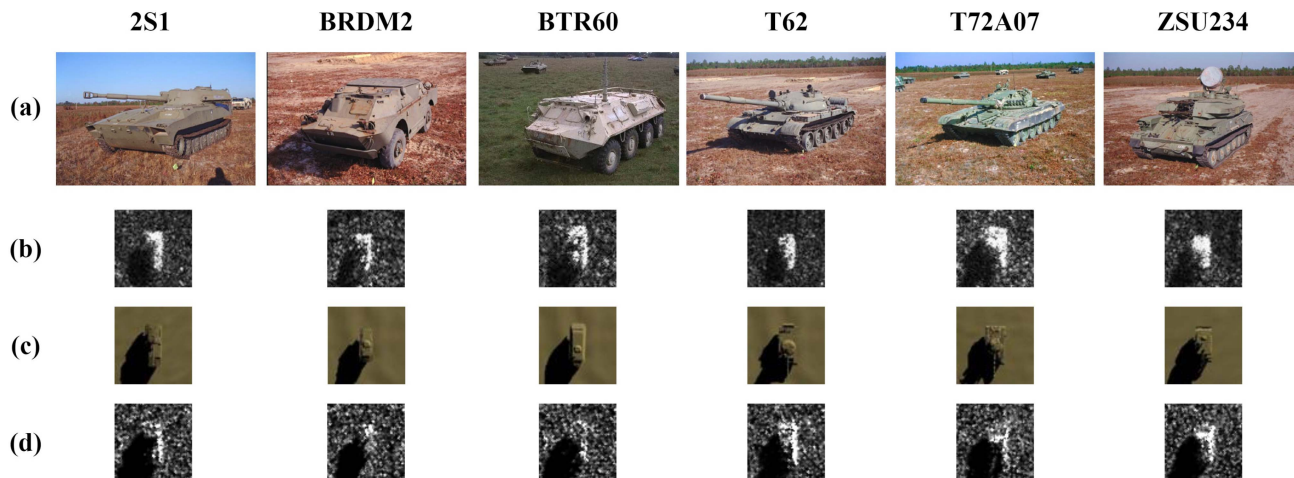
Fig. 4. Example images of six military equipment from different datasets. (a) Real photos. (b) Real SAR images. (c) Optical images given by rendering. (d) Simulated SAR images. Photos in (a) are provided in MSTAR dataset website [29]. For images in (b), (c), and (d), the azimuth angle is 144^\circ and depression angle is 15^\circ .
