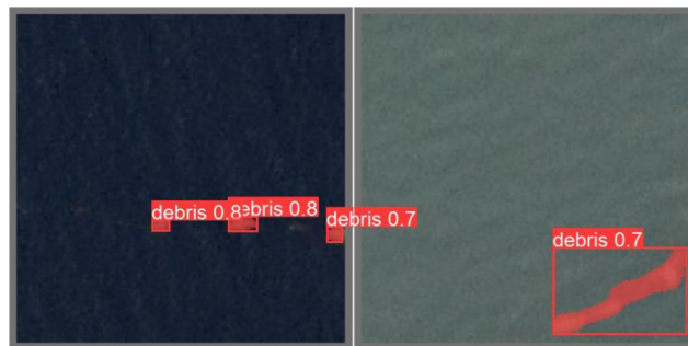
Fig. 1. Example of an instance segmentation model applied to drone imagery. This shows that the AI was able to identify the litter scattered on the ocean.
