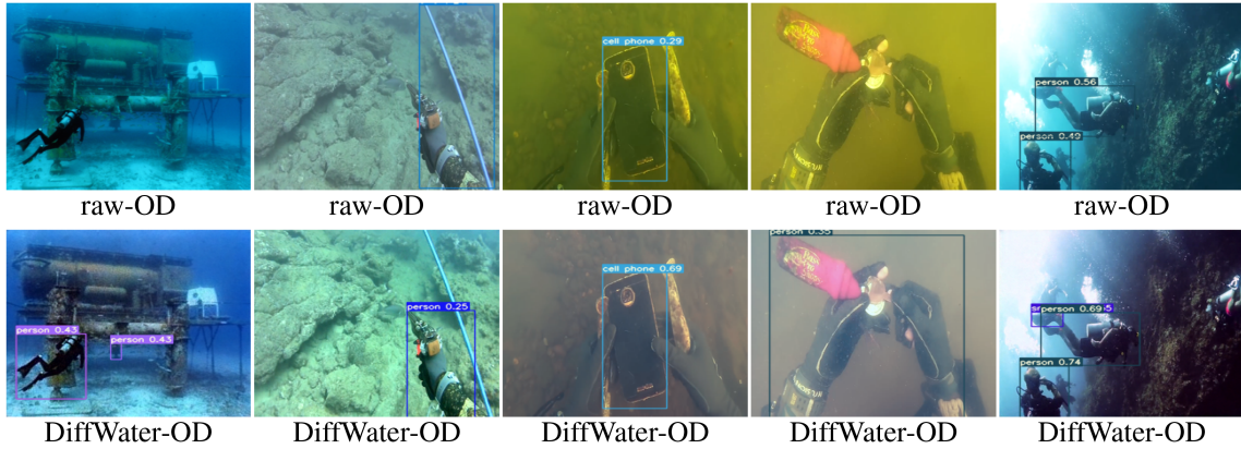
Fig. 11. Effect of DiffWater for OD on input and enhanced images. (Top) The above figure shows the YOLOv7 OD result of the input image. (Bottom) The bottom is the target detection result of YOLOv7 enhanced by DiffWater.
