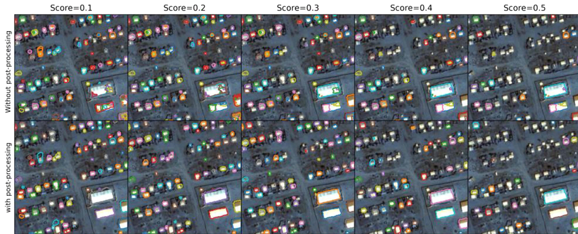
Fig. 12. Output sensitivity for modified score threshold (objectness score) and role of postprocessing. Results are taken from transfers Kutupalong-2017 \rightarrow Minawao-2017 using the MMD domain approach.
