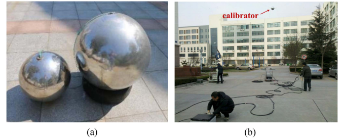
Fig. 2. Photograph of (a) calibrator and (b) measurement for noise background level.
