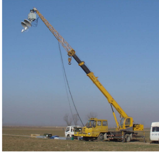
Fig. 1. Photograph of the truck-mounted scatterometer system.
