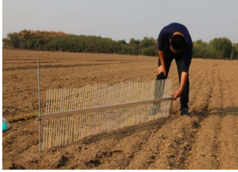
Fig. 4. Photograph of a roughness profile with a 2.4-m-long needle profilometer and a 3-cm interval between needles.
