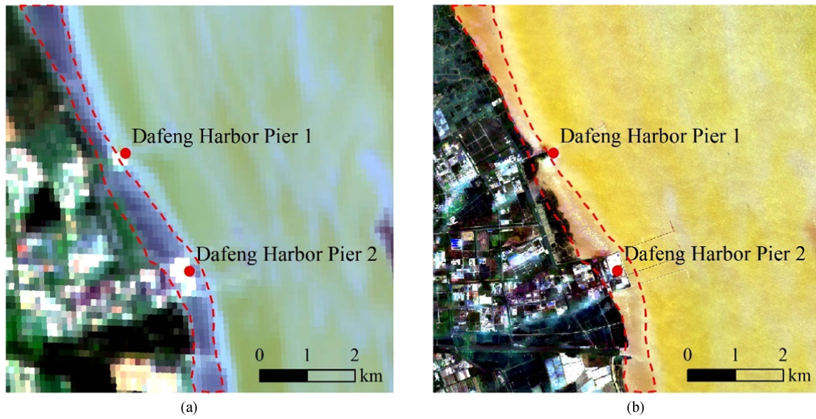
Fig. 5. Moments of high tide when intertidal zones are exposed. (a) Represents the moment of high tide captured by GOCI-II. (b) Represents the moment of high tide captured by the fusion image. The red polygon indicates the intertidal zone.
