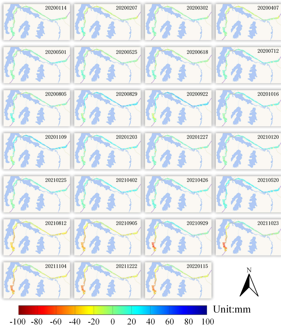
Fig. 10. Time-series deformation results over the study area.
