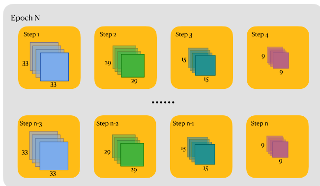
Fig. 9. Sample strategy of custom data loader. In this diagram, the yellow blocks depict the steps within an epoch. The blue, green, turquoise, and pink squares represent the HSI samples of varying sizes. Each sample encompasses a set of pixels centered around the target pixel.
