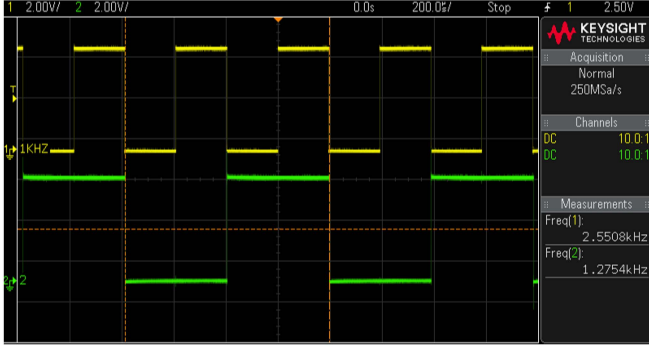
Fig. 5. Checking the frequency component applied to the LED using the oscilloscope.
