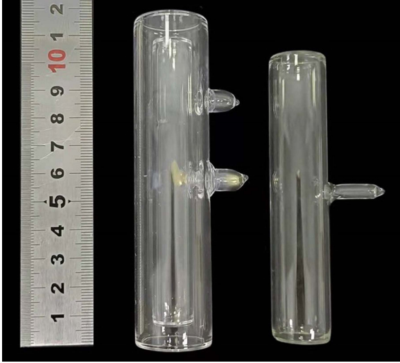
Fig. 2. Double-layer vapor cell (left) and the single-layer vapor cell (right). The double-layer atomic vapor cell has a vacuum space between two layers of quartz glass, effectively reducing the thermal conduction between the vapor cell and the ambient air. The length and the diameter of the double-layer vapor cell are 11 cm and 2.6 cm, respectively. The length and the diameter of the single-layer vapor cell are 10 cm and 2 cm, respectively.
