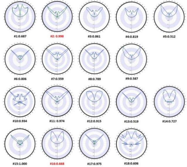
Fig. 17. Intensity distribution for L_{18} experiments.
