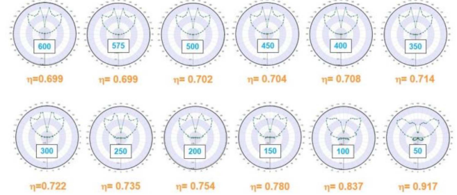
Fig. 12. Effect of sapphire length ( L = 600\text{--}50 \mu\text{m} ) on intensity distribution.
