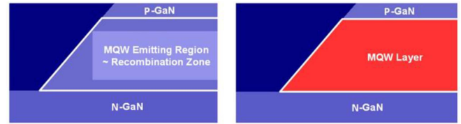
Fig. 4. Modeling of MQW layer: Emitting region (photon source) is immersed in MQW layer.
