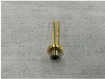
Fig. 11. TO-56 package appearance.
