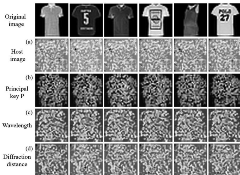
Fig. 6. Retrieved images with the incorrect keys in the decryption process: (a) Incorrect host image; (b) Incorrect random phase mask; (c) the wavelength is 600 nm; and (d) the diffraction distance of the host image has an error of 5%.
