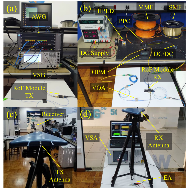
Fig. 3. Photographs of the experimental setup: (a) RoF transmitter; (b) RoF receiver and PoF link; (c) 10-m wireless indoor link; (d) indoor receiver side.
