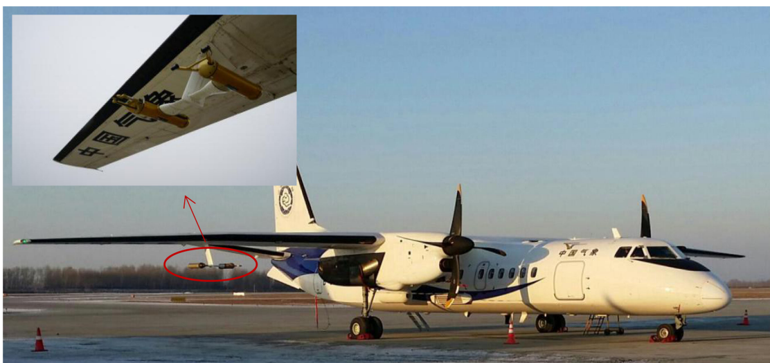
Fig. 4. The Aircraft Xinzhou 60 and detection equipment.
