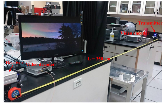
Fig. 5. Experimental setup of a free-space optical link used for transmission of digital video signals at a 350-cm-long propagation distance.
