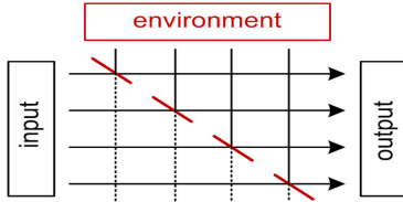
Fig. 6. A schematic of the model of lossy Bosonic channel.
