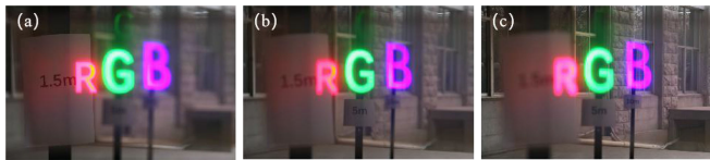
Fig. 9. (a), (b) and (c) are the display effects when the camera focuses on the three letters R, G and B at different distances.
