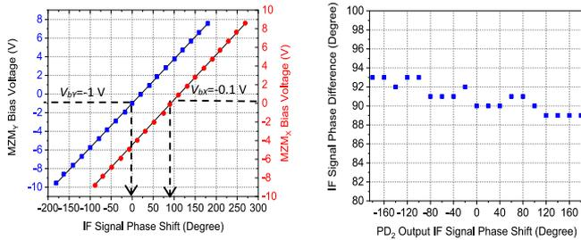
Fig. 7. (a) Predicted (solid line) and measured MZM<sub>X</sub> (red dots) and MZM<sub>Y</sub> (blue squares) bias voltage versus the phase of PD<sub>1</sub> and PD<sub>2</sub> output IF signal relative to the reference IF signal phase. (b) PD<sub>1</sub> and PD<sub>2</sub> output IF signal phase difference for different PD<sub>2</sub> output IF signal phases obtained by adjusting MZM<sub>X</sub> and MZM<sub>Y</sub> bias voltages shown in (a).
