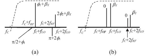
Fig. 2. Spectra of the optical signals into (a) PD<sub>1</sub> and (b) PD<sub>2</sub>. Magnitude response of the OBPF (dashed line).  $f_c$ : optical carrier frequency,  $f_{RF}$ : RF signal frequency,  $f_{LO}$ : LO frequency.
