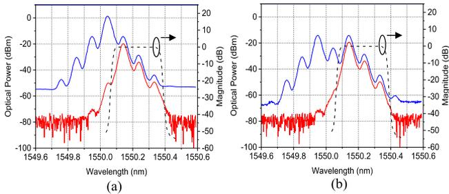
Fig. 4. Normalised magnitude response of OBPF<sub>1</sub> (dashed line) and measured optical spectrum before (blue line) and after (red line) OBPF<sub>1</sub> when both MZM<sub>X</sub> and MZM<sub>Y</sub> are operating at (a) the peak bias point and (b) the null bias point.
