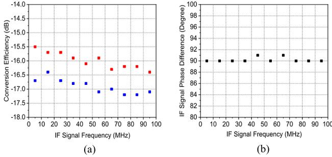
Fig. 9. (a) Measured I/Q mixer conversion efficiency at PD<sub>1</sub> output (red square) and PD<sub>2</sub> output (blue square) for different IF signal frequencies. (b) Measured IF signal phase difference for different IF signal frequencies.
