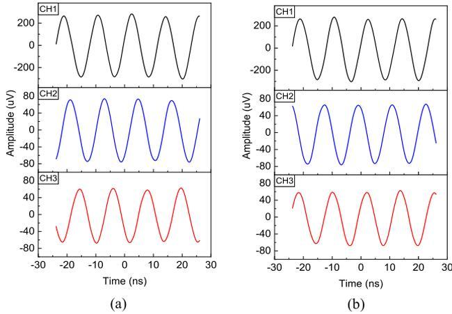
Fig. 6. IF signal waveforms measured at PD<sub>1</sub> (middle trace) and PD<sub>2</sub> (bottom trace) output when both MZM<sub>X</sub> and MZM<sub>Y</sub> are biased at (a) the peak point and (b) the null point. A reference IF signal waveform measured at the electrical mixer output is shown in the top trace.
