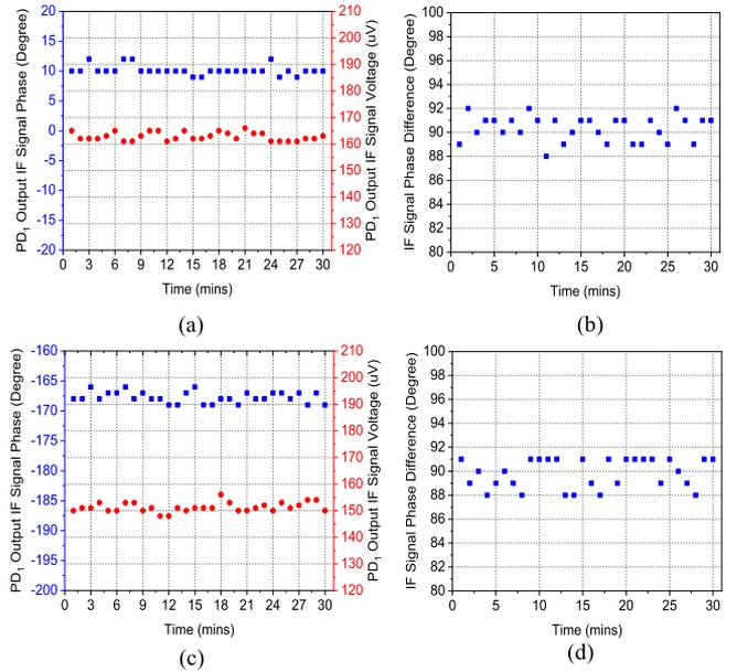
Fig. 11. Stability measurement of PD<sub>1</sub> output IF signal phase relative to the reference IF signal phase (blue square) and PD<sub>1</sub> output IF signal peak-to-peak voltage (red square), and stability measurement of the two output IF signal phase difference, when both MZM<sub>X</sub> and MZM<sub>Y</sub> are biased at the peak point ((a), (b)) and the null point ((c), (d)).
