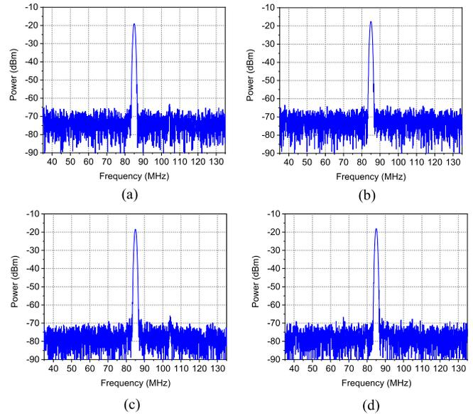
Fig. 5. Measured electrical spectra at the I/Q mixer (a) PD<sub>1</sub> and (b) PD<sub>2</sub> output when both MZM<sub>X</sub> and MZM<sub>Y</sub> are biased at the peak point. Measured electrical spectra at the I/Q mixer (c) PD<sub>1</sub> and (d) PD<sub>2</sub> output when both MZM<sub>X</sub> and MZM<sub>Y</sub> are biased at the null point.
