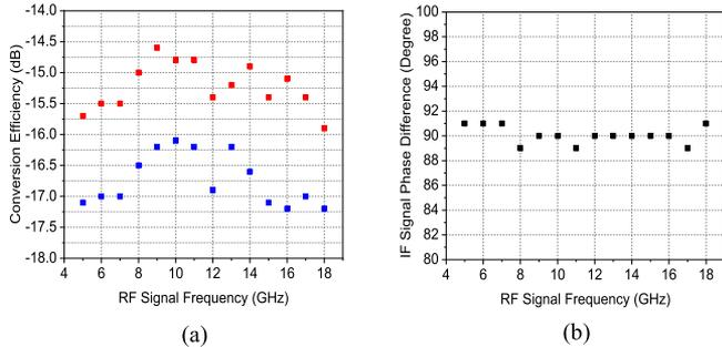
Fig. 10. (a) Measured I/Q mixer conversion efficiency at PD<sub>1</sub> output (red square) and PD<sub>2</sub> output (blue square) for different RF signal frequencies. (b) Measured IF signal phase difference for different RF signal frequencies.
