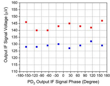
Fig. 8. PD<sub>1</sub> (red square) and PD<sub>2</sub> (blue square) output IF signal peak-to-peak voltages for different PD<sub>2</sub> output IF signal phases.
