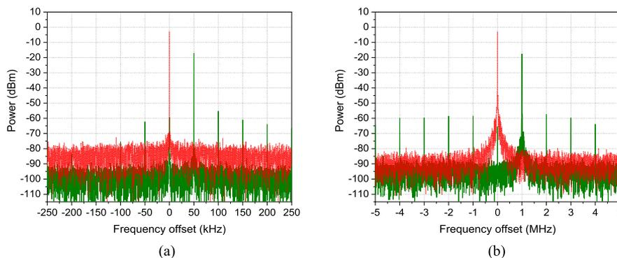
Fig. 5. DP-DDMZM based frequency translator input (red dashed line) and output (green line) electrical spectrum for a sawtooth wave with a frequency of (a) 50 kHz and (b) 1 MHz, into DDMZM<sub>1</sub>. The frequency translator input microwave signal frequency is 10 GHz.
