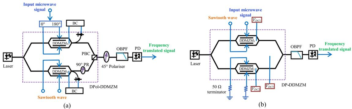
Fig. 1. Structures of the new microwave photonic frequency translator based on (a) a DPoL-DDMZM and (b) a DP-DDMZM.
