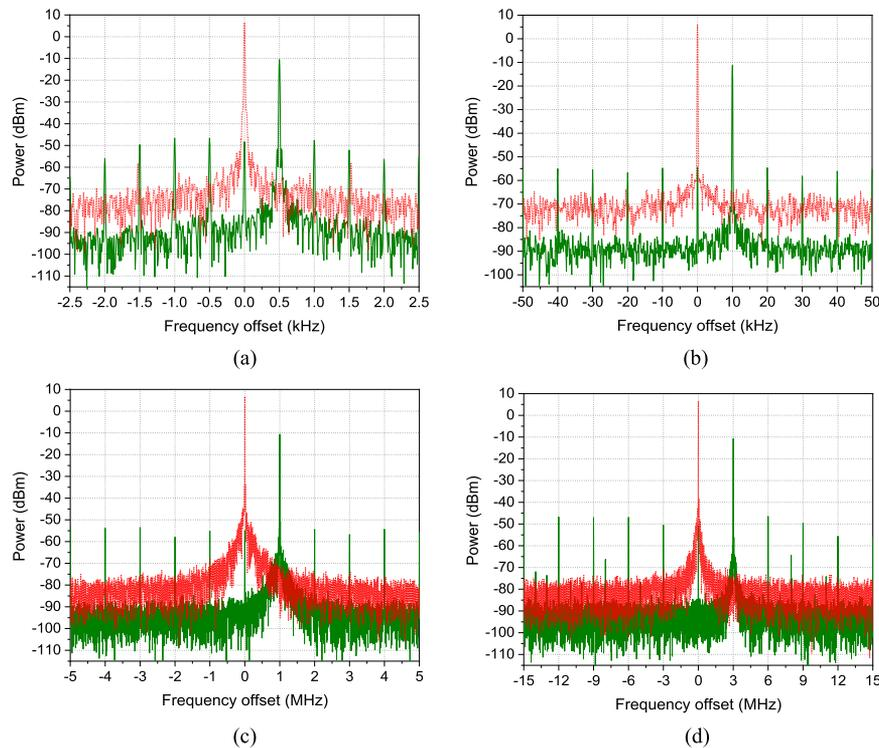
Fig. 2. DPoL-DDMZM based frequency translator output electrical spectrum (green line) for sawtooth waves with a frequency of (a) 500 Hz, (b) 10 kHz, (c) 1 MHz and (d) 3 MHz, into DDMZM<sub>Y</sub>. Electrical spectrum (red dashed line) of the 12 GHz microwave signal into DDMZM<sub>X</sub>.
