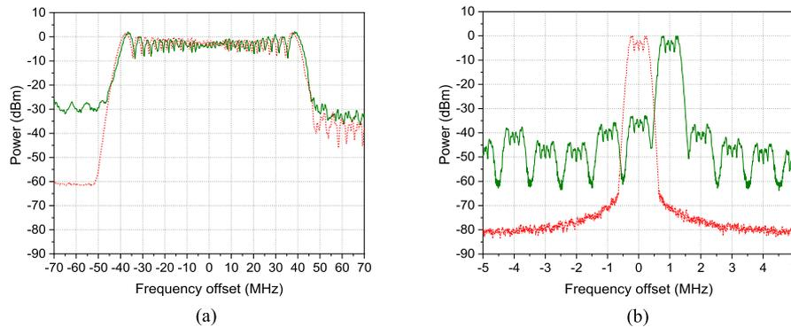
Fig. 4. Electrical spectrum of a FMCW signal at 5.88 GHz into the DPoL-DDMZM based frequency translator (red dashed line) and frequency translator output electrical spectrum (green line) when the FMCW signal has a (a) 40 MHz and (b) 200 kHz frequency deviation.
