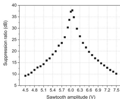
Fig. 6. DP-DDMZM based frequency translator spurious suppression ratio versus the sawtooth wave amplitude.
