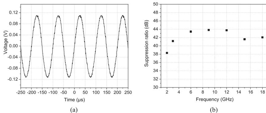
Fig. 3. (a) Waveform of the 12 GHz + 10 kHz frequency translated microwave signal after down converted to 10 kHz via a mixer. (b) Spurious suppression ratio of the DPoL-DDMZM based frequency translator operating at different input microwave signal frequencies.
