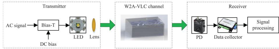
Fig. 2. The block diagram of a laboratory W2A-VLC system.
