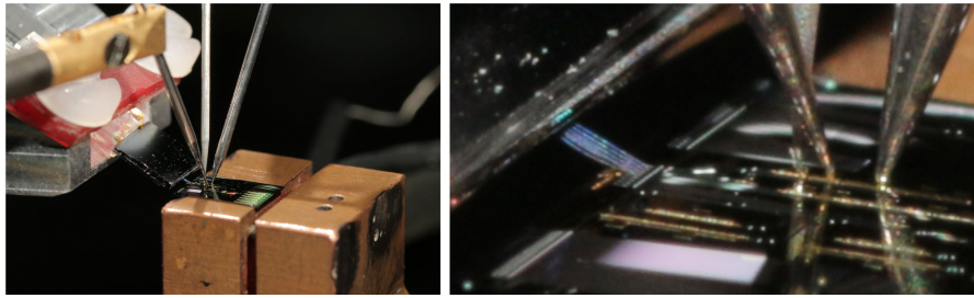
Fig. 14. (left) View of fingers landed on sample for performing the SOA gain measurements. (right) Zoomed-in view showing the fingers at the probe tip.
