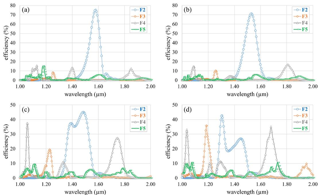
Fig. 2. Light coupling efficiencies for grating structures with unit cells  $F_2$ ,  $F_3$ ,  $F_4$ , and  $F_5$  with an etch – depth = 70 nm for (a)  $\theta = 6^\circ$  and (b)  $\theta = 10^\circ$ . Results for  $\theta = 10^\circ$  with different etch – depths are also plotted for (c) etch – depth = 110 nm and (d) etch – depth = 140 nm.
