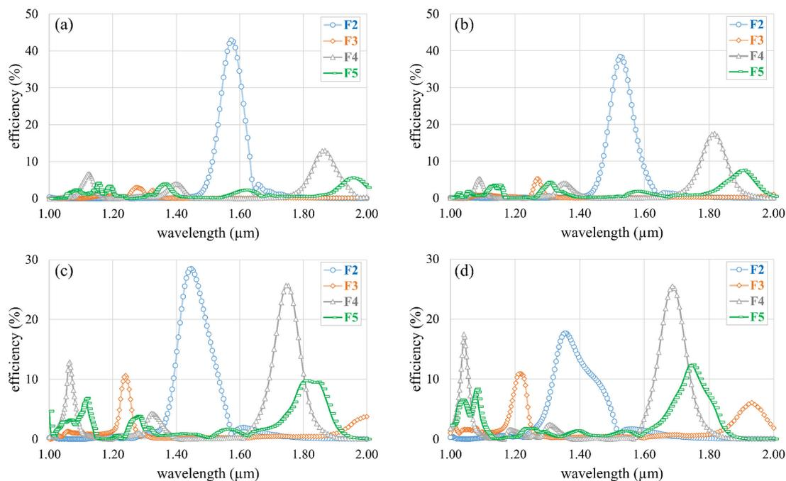
Fig. 4. Light coupling efficiencies for grating structures without the bottom-gold mirror layer, with unit cells  $F_2$ ,  $F_3$ ,  $F_4$ , and  $F_5$  with an etch – depth = 70 nm for (a)  $\theta = 6^\circ$  and (b)  $\theta = 10^\circ$ . Results for  $\theta = 10^\circ$  with different etch-depths are also plotted for (c) etch – depth = 110 nm and (d) etch – depth = 140 nm.
