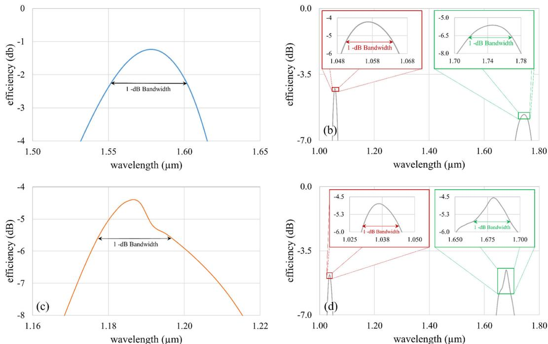
Fig. 3. Light coupling efficiencies with the corresponding 1-dB bandwidths for grating structures with unit cells  $F_2$ ,  $F_3$ , and  $F_4$ . Results are for (a)  $F_2$  with  $\theta = 6^\circ$  and etch – depth = 70 nm, (b)  $F_4$  for  $\theta = 10^\circ$  and etch – depth = 110 nm, (c)  $F_3$  for  $\theta = 10^\circ$  and etch – depth = 140 nm and (d)  $F_4$  for  $\theta = 10^\circ$  and etch – depth = 140 nm.
