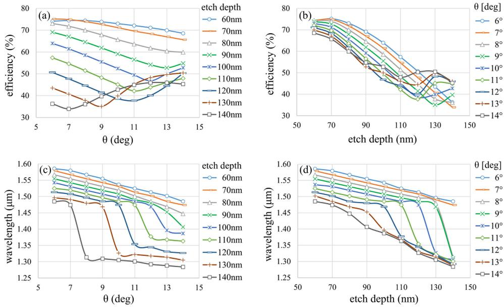
Fig. 5. Highest coupling efficiency for the  $F_2$  system consisting in the repetition of 24 periods  $AB$ , as a function of a) fiber's tilt-angle and b) groove etch-depth. c) and d) show the wavelengths associated with these coupling efficiency peaks as a function of the fiber's tilt-angle and groove etch-depth, respectively. Small losses for  $\theta = 6^\circ$  and etch - depth = 70 nm in a) are mainly due to undesired reflections at the grating-fiber interface (see **Visualization 1**).
