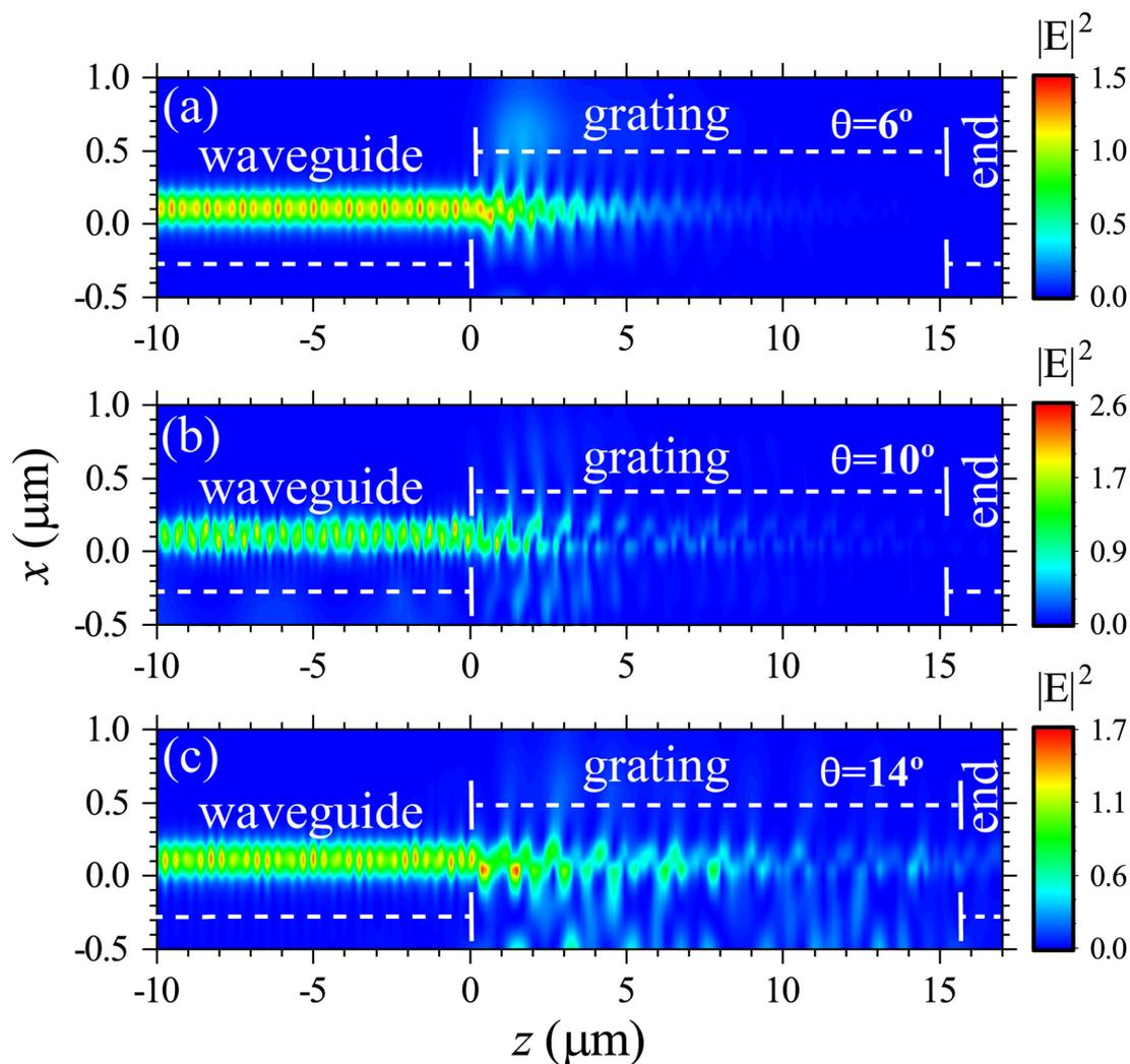
Fig. 8. Field profiles associated with the maximum CE peaks for (a)  $F_2$ , (b)  $F_3$ , (c)  $F_4$ , results were calculated for  $\theta = 6^\circ$ ,  $\theta = 10^\circ$ , and  $\theta = 14^\circ$ , respectively. The waveguide thickness was 220 nm. Different etch-depths were used for each Fibonacci step: (a) 70 nm, (b) 140 nm, and (c) 140 nm.
