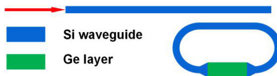
Fig. 1. The waveguide structure diagram of the Ge-on-Si microring photodetector, in which the germanium absorption layer is on the silicon waveguide.
