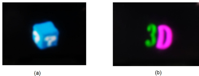
Fig. 11. 3D image reconstructed by the mono-view integral imaging system: (a) 3D image of 3D scene 1 and (b) 3D images of 3D scene 2.
