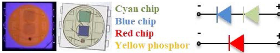
Fig. 3. A full-spectrum white LED package.
