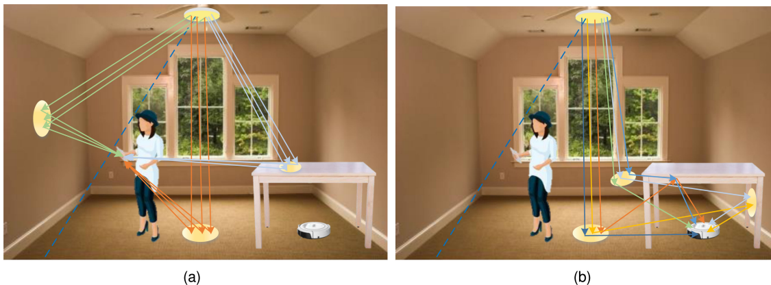
Fig. 1. Examples on the NLOS VLC link. (a) The first-order reflection from the LED to the hand-held terminal. (b) The second-order reflection from the LED to the robot under the table.
