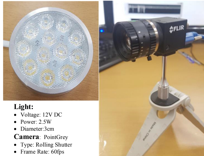
Fig. 5. The device for SNR measurement.
