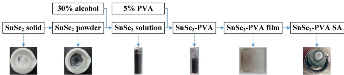
Fig. 1. Preparation flow diagram of SnSe 2 -PVA SA.
