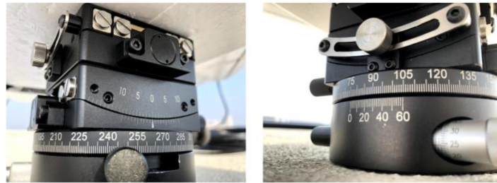
Fig. 5. The three-dimensional turn table instrument used as reference rotation angles.
