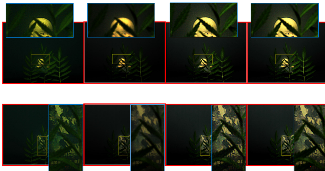
Fig. 6. The recovered images by different methods, from left to right: UDCP, traditional polarized-difference dehazing (PD), our polarized-difference dehazing, Synthetic aperture dehazing.
