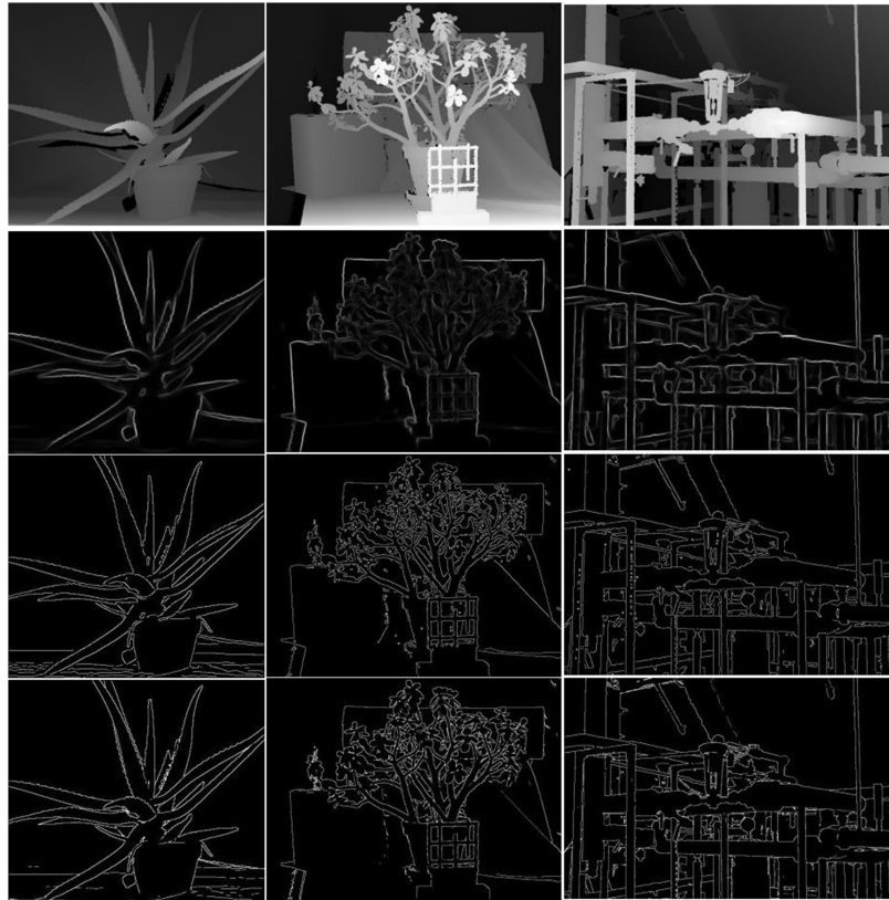
Fig. 9. Edge detection results on depth images with high resolutions. The first rows are depth images with high resolutions, and the other rows are edge detection results by SE-MS, Canny, and the proposed method.
